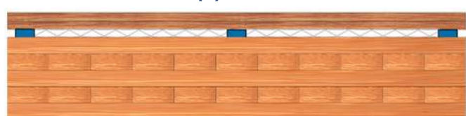
1" PAC-IFB with 5-ply Cross Laminated Timber
