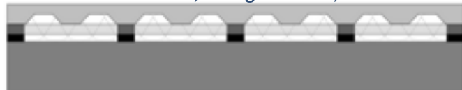
2" PAC-IFB with track, corrugated deck, and concrete
