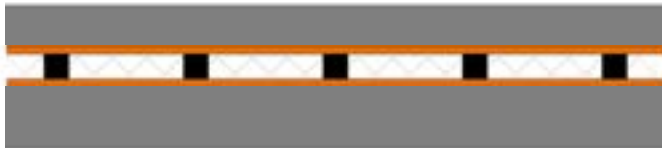
2" PAC-IFB with track, corrugated deck, and concrete
