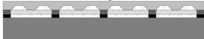
2" PAC-IFB with track, corrugated deck, and concrete
