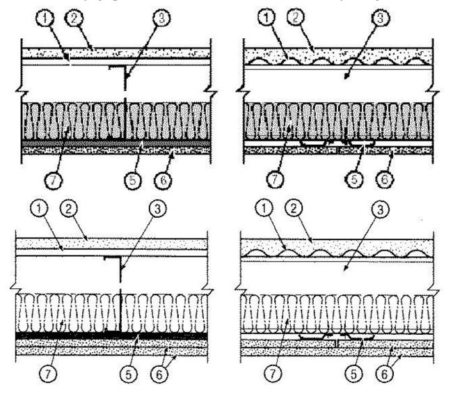
1. **Steel Deck** — Min 9/16 in. deep, 22 MSG galv corrugated fluted steel deck. Overlapped one corrugation at each side and attached to each joist with 5/8 in. long No. 10-16 TEK screws at each side joint and no more than 12 in. OC between sides.
