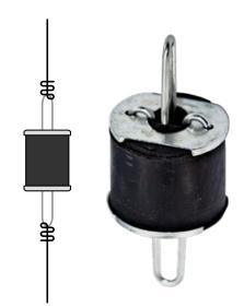
The **RSIC-WHI** is designed for use with any wood, steel or concrete application where a dropped drywall ceiling is required. The RSIC-WHI isolator installed mid-wire between the structure and a drywall grid ceiling, or CRC and hat channel ceiling. The RSIC-WHI Isolator has acoustical design load ratings of 30, 50, 70, 100, 145, and 220 lbs per isolator. The RSIC-WHI is designed to work within a range between 50% and 100% of the published acoustical design load.
