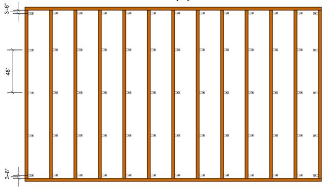
RSIC-1 Low Profile installed on Joist 16" o.c. for 1 or 2 layers of 5/8" gypsum board RSIC-1 Low Profile Clips spaced at 16" x 48"
