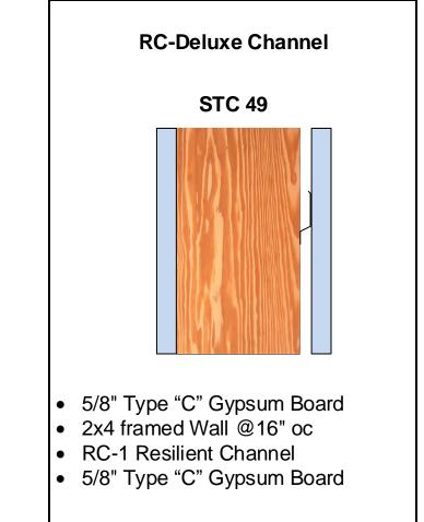
Tested and Approved Resilient Channels: **Dietrich** RC-1 pro, **Cemco** RC-1, **Phillips** RC-1 Select (Tru-25), **Phillips** RC-1 Max, **Marino Ware** RC-1, **Marino Ware** Rc-Max, **Scafco** Serenity RC-Plus.
